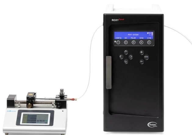
Fig. 2. ROXY Exceed EC with syringe pump.
