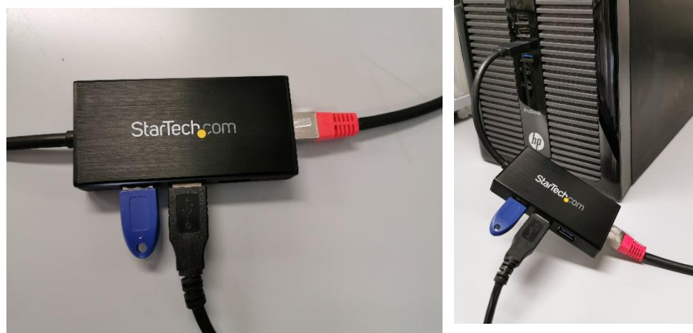
Fig. 4. Example of LAN adapter connections and LAN adapter connected to the PC.
