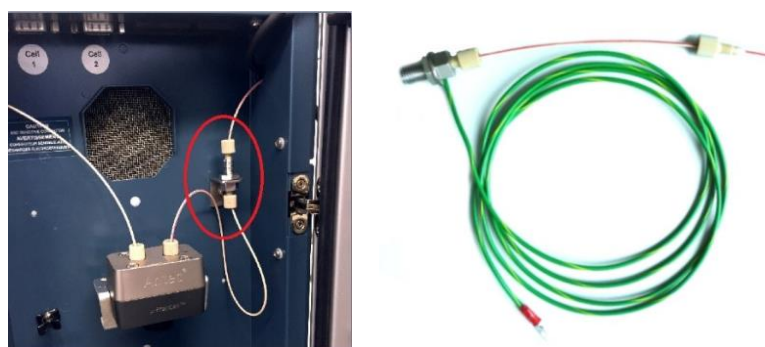
Fig. 7. The grounding kit inside the ROXY Exceed (left) or for external use (right).
